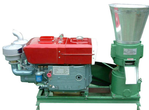
Small Flat Die Pellet Mill Powered By A Diesel Engine
