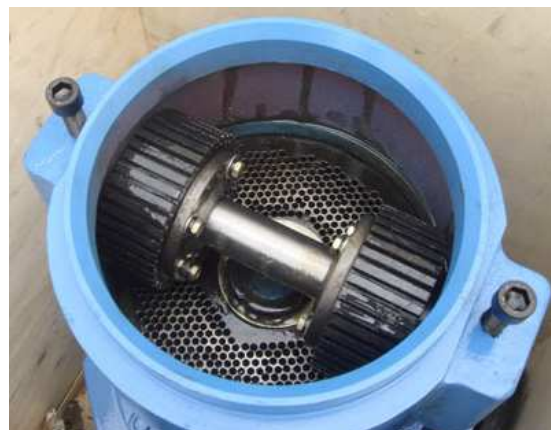
The Die and Roller of the PK/KL Pellet Mill
